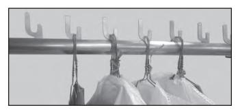
"STEP" PENDANT CHAIN - designed to transport bundled or single hangered goods with minimal sliding friction and/or hanger wear. By keeping single or bundled goods off the track and carried on the pendant arm, longer conveyor designs are possible.
