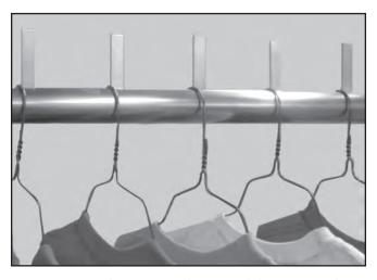
**PENDANT UP CHAIN** - this 3-1/8" pendant spaced chain is primarily used for garment finishers and single garment transport.
