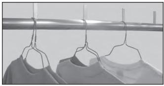
**PENDANT UP CHAIN** - this 6-1/4" spaced pendant chain is used primarily for hangered goods. The small diameter tube allows hangers to be hung directly on the track and pushed by the pendant. Loading and plowoff anywhere along the conveyer system.
